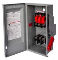
Siemens Low Voltage Circuit Protection Heavy Duty Safety Switches. Type: ENCLOSED, SAFETY SWITCH Special Features: N/A Std: UL V. Rating: 600VDC A. Rating: 200A No. Of Poles: 3P F. Rating: 60Hz Action: SINGLE THROW Closed Contact Resistance: N/A Connection: N/A
